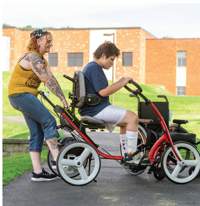
The seat glides up and down on a low-friction rail. This rider pushes with his feet to help his caregiver raise the seat.
